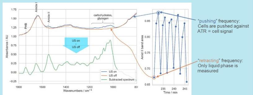
Figure 6: Selective measurement of the bacteria and the carrier liquid by soniccatch (2) and an ATR-FTIR probe (3): the cells, producing PHB (5) are pressed to the ATR-Element (4) respectively.
