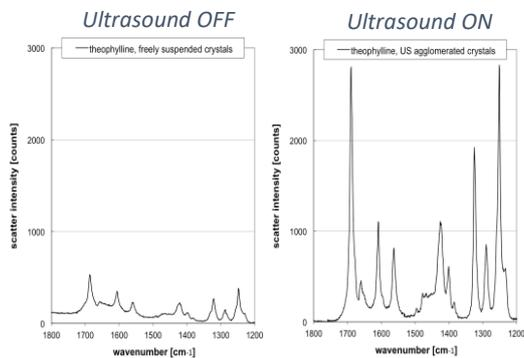
Figure 3: Theophylline crystals. Raman- Signal enhanced with ultrasound particle agglomeration, also see figure 4
