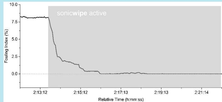
Figure 9: Removal of a biofilm (fermenting yeast cells) from an in-line sensor's window by applying ultrasound (left without and right with ultrasound).
