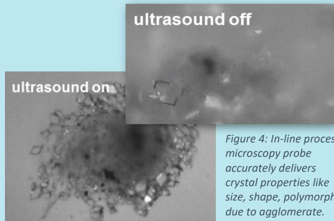
Figure 4: In-line process microscopy probe accurately delivers crystal properties like size, shape, polymorph due to agglomerate.
