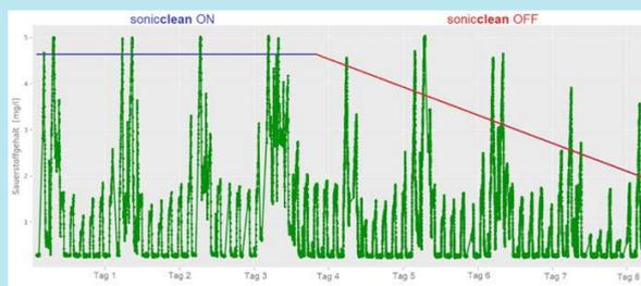
Figure 10: sonicclean keeps the O<sub>2</sub>-levels stable, as the sensor is not affected by layers. The aeration is otherwise activated too often due to falsified O<sub>2</sub>-levels, causing unnecessary energy loss and process technological difficulties.
