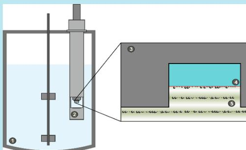
Figure 5: Cyanos produce PHB through sunlight and CO<sub>2</sub> in a 5 l bioreactor (1), PHB is accumulated inside the cell.
