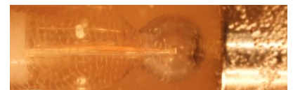
Figure 2: Making the ultrasound field visible with the help of suspended particles: the pattern they form on the pH-probe reassembles the ultrasound force's active area and indicates the range of the cleaning effect
