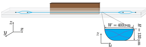
Figure 1: Sketch of the acoustophoresis glass chips (light gray) with a dimension of 70 \times 3 \times 1.1 mm 3 . The long-straight microchannel (light blue) has a dimension of 45 \times 0.403 (at its top) \times 0.133 mm 3 . The piezoelectric transducer (brown) was mounted to the side of the chip. The half-wave standing-wave field is indicated by the dashed magenta lines.
