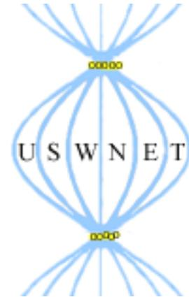
Ultrasonic standing-wave (USW) radiation forces can be used for particle manipulation, separation and enrichment. We have developed two different miniaturized USW systems, a microtiter plate USW system and a lab-on-chip USW system. The goal is to use the devices for ultrasensitive biochemical analysis and for gentle handling of single cells in microchannels.
